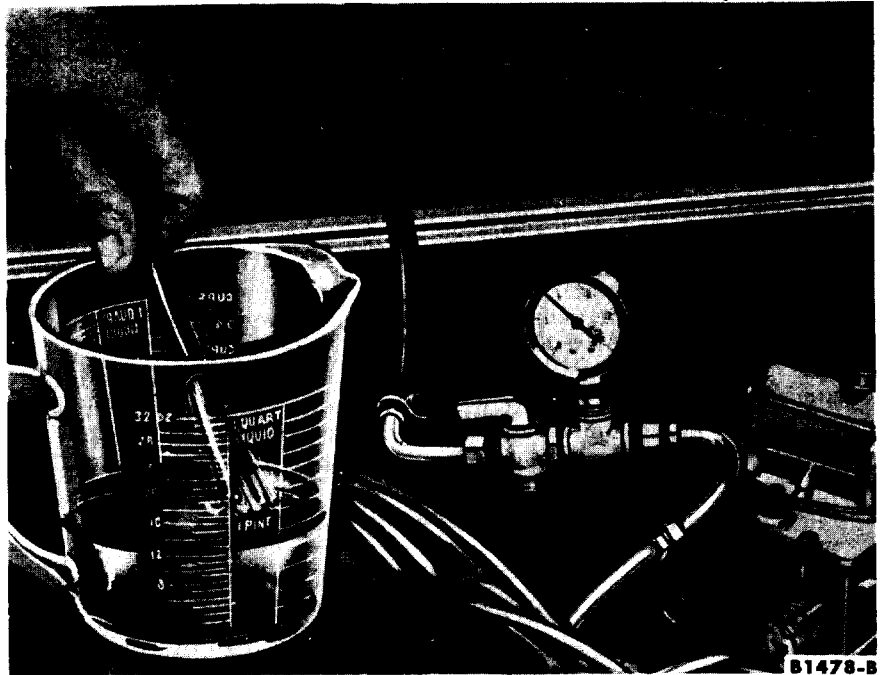
FIG. 2—Fuel Pump Pressure and Capacity
