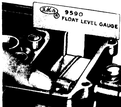
FLOAT SHOULD JUST TOUCH AT THIS POINT
