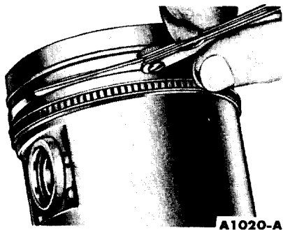
FIG. 69—Ring Side Clearance
