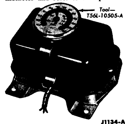
FIG. 13—Voltage Regulation Setting Thermometer
