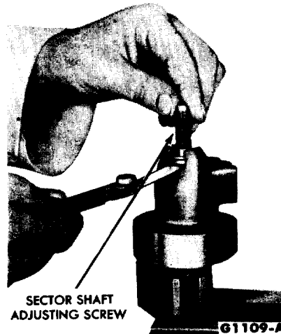
FIG. 23—Adjusting Screw Clearance Check
