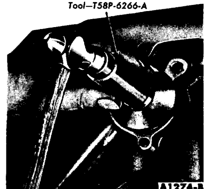
FIG. 83—Camshaft Rear Bearing Bore Plug Installation
