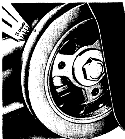
SEE SPECIFICATIONS FOR IGNITION TIMING SETTINGS B1209-B FIG. 16—Timing Marks
